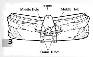
Position the ends of the frame tubes against the middle holes in a frame.
